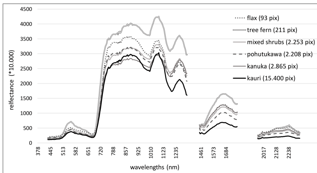
Figure 7. Mean spectra of kauri (black) and five other canopy species (grey) that have the highest separabilities from the kauri spectrum in this study (see Table A2). The number of pixels (pix) used to generate the mean spectra is given in parentheses.
