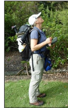
Photo: Single tree mapping with a Bluetooth GPS on a hiking stick in the backpack, connected to QGIS maps on a tablet with aerial images and crown height model.
