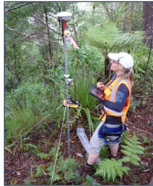
Photo: Centre station for circular sample plots with GPS, compass and vertex transponder.
